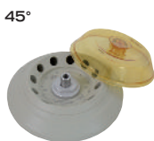
Angle rotor, 12-place Cat. No. 01252-A n= 14,000 min -1 , max RCF 15,558
