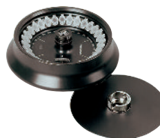
Angle rotor, Cat. No. 01689-A 30-place, n= 14,000 min -1 max RCF 21,255
