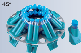
Angle rotor, Cat. No. 01418 8-place N = 4.500 min -1 max. RCF 3,305 illustrated with adapters 01467
