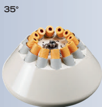
Angle rotor, Cat. No. 01620A 6-place, n= 9,000 min -1 , max. RCF 9,418. illustrated with adapter set 01646
