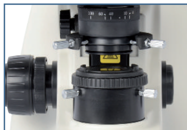
KOEHLER ILLUMINATION / SLIDING-IN ABBE BRIGHT FIELD CONDENSER
